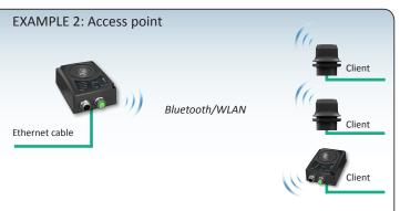
The Wireless Bridge can act as an access point connecting up to seven different clients. This example shows connection to several Anybus Wireless Bolts and one Wireless Bridge. The Anybus Wireless Bridge and Bolt work seamlessly together.
