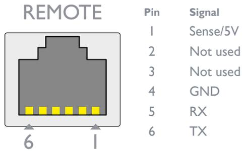
*Note: The TX detects presence of an incoming power signal to determine whether 5V should be supplied at the RX.*
