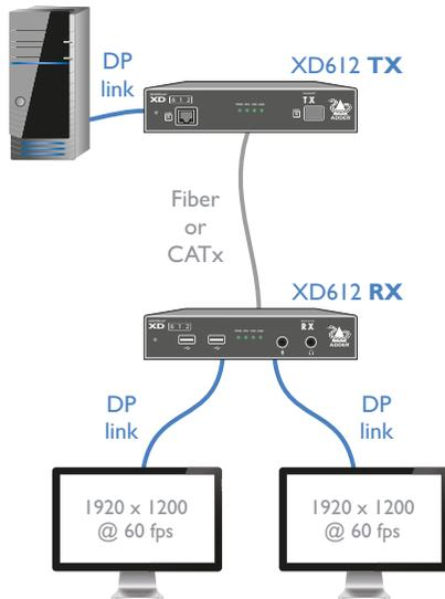
The video displays do not need to be MST-compliant and no hub is required.
