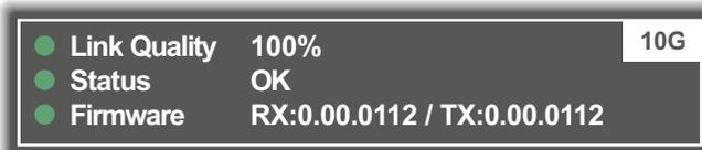
The example above shows a configuration that is working correctly. If the communication link was working correctly, but the video signal was lost, it might report as follows:
