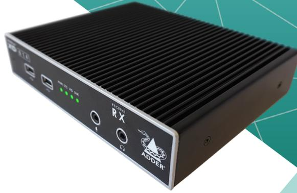
A high-resolution quad-head KVM extender. High definition video, USB2.0 and audio are transmitted on a single CATx or fiber cable.
