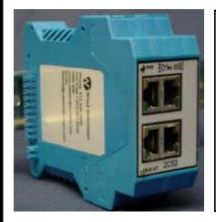
The 2C53 Ethernet, 10/100 Base-T(X), Unmanaged Switch Module requires no user configuration. The four RJ45 ports will automatically negotiate data rates and will auto-sense Full or Half duplex operation. The 2C53 will automatically learn the addresses of the devices connected to each port (up to 1024) and will buffer and route messages accordingly.
