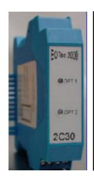
The Patented 2C30 Self-Healing Ring Module provides fiber media redundancy when utilized in each node or drop of a fiber optic ring-network. The 2C30 device detects and redirects data to the secondary fiber path when a break in the fiber occurs between two adjacent nodes. The 2C30 automatically resets when the fiber path has been restored. Visible LED indicators in conjunction with relay contacts provided local and remote monitoring of the integrity of the fiber optic network.
