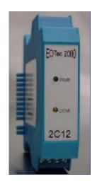
The 2C12 Module provides electrical interface for Allen-Bradley Data Highway, Data Highway Plus and Remote I/O networks by conditioning the electrical signals supplied to and from the Allen-Bradley equipment for transmission over the fiber optic network.
