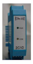
The 2C10 Module provides RS-232 or RS-485 communications protocol electrical interface conditioning for data transmission over the fiber optic network. The module can be selected to support either point-to-point RS-232 or multi-drop RS-485 half-duplex communications.
