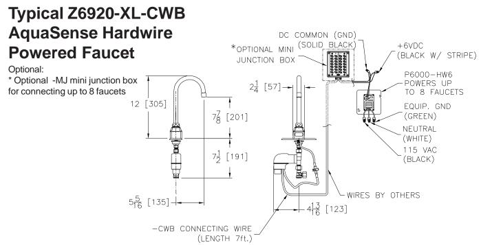
NOTE: MUST USE EITHER ZURN P6000-HW6 HARDWIRE POWER CONVERTER OR ZURN P6900-ACA PLUG-IN POWER CONVERTER TO ENSURE PROPER OPERATION. USING A POWER CONVERTER OTHER THAN ZURN MAY RESULT IN OPERATION MALFUNCTION OR UNIT FAILURE.
