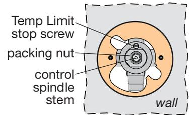
Figure 3 Valve adjustments
