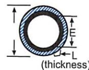
Comes standard as 300 series stainless steel washer with Buna inner ring. Also available with Viton® ring or as a stainless steel washer with Viton® ring. Add -V for Viton® or -SS-V for stainless steel/ Viton®
