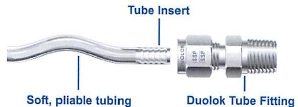
In general, Duolok tube fittings may be used with a variety of plastic tube materials without any special preparations. However, very soft-wall, pliable tubing such as Tygon® needs a tube insert for support prior to insertion in the Duolok tube fitting. The standard Duolok tube fitting installation instructions (see page 6) are then followed for proper make-up.
