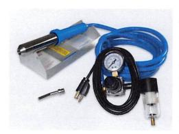
The Model 63 SI-1005 Welder comes with a standard 500 watt 120 volt Element, air Filter, Gauge, Regulator, Round Tip, Tray and Welder Guide CD. The SI-1005 is considered one of Seelye's work horse welders. This is an ideal welder for small repairs or first time users. This welder ranges from ambient up to 900° F (maximum temp. reached when used with a 650 watt Element).
