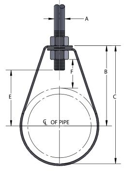
"E" dimension includes exposed rod threads beyond bottom of the hex nut. Exposed rod thread dimension is equal to the diameter of the rod used.
