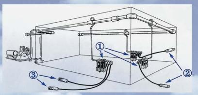
La-Man provides a wide range of compressed air filtration and preparation devices. As shown, the Extractor/Dryer 1 is installed for primary filtration and moisture removal. Each unit is augmented with either the Pneuguard® Inline Dryer 2 or Dryer/Pneuguard® 3 for additional filtration.
