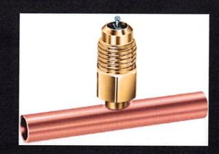
Our copper braze tees can be bent, cut, flared, swaged, or pinched. The extra depth slip fit braze cups provide simple installation anywhere along the line. Use Sil-phos alloy.
