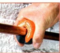
This is a great tool to have when you don't have enough swing room to use a full size tubing cutter. You can cut copper tubing with less than one inch of clearance. And it's ideal for stub-out work.
