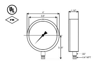
Application: Fluid medium which does not clog connection port or corrode copper alloy.
