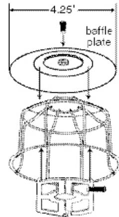
Designed to provide protection against low level impacts to the sprinkler head. Features a cage and clamping base plate. This design can provide additional protection for sprinklers that may experience greater opportunity for repeated abuse. Caution: Head guards will not protect sprinkler heads from severe abuse or impact.
