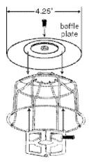
Designed to provide protection against low level impacts to the sprinkler head. Features a cage and clamping base plate. This design can provide additional protection for sprinklers that may experience greater opportunity for repeated abuse.
