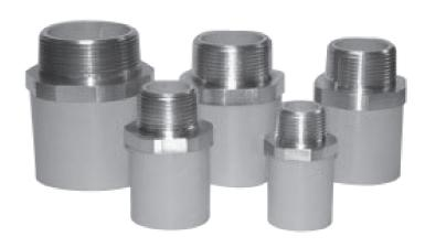
Spears® revolutionary design features a special molded-inplace brass male thread that is fully lined with CPVC for superior corrosion resistance. Available in sizes 3/4" through 2"
