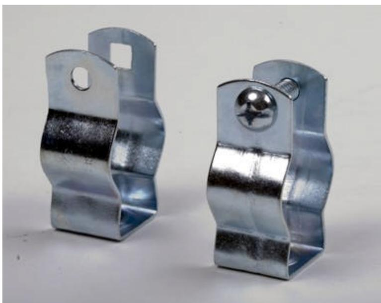
Stamped from heavy gauge steel with smooth edges. Hole on top can accept a 1/4" bolt or screw. Conduit hangers are available with or without bolt assembly. Zinc Plated to resist corrosion
