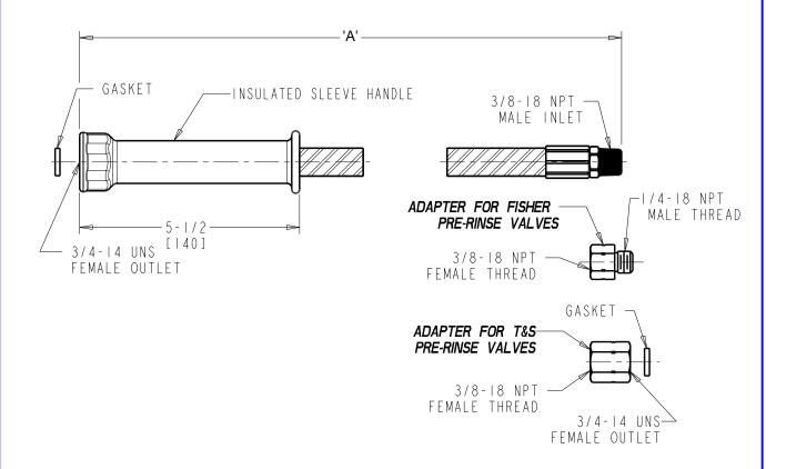
DIMENSIONS ARE IN INCHES AND [MILLIMETERS].
