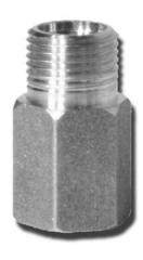
Designed to be used as sprinkler head extensions when a drop nipple length has been cut too short or when the finished ceiling has changed from its intended location. Using the appropriate length extension will allow for realignment of the sprinkler head without removing and recutting the drop nipple.
