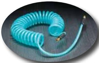
**Note:** Each length of assembled tubing or hose includes a 4" pigtail and a 20" whip end, assembled to 1/4" or optional 3/8" (priced upon request) male NPT permanent crimped swivel brass fittings with rubber bend restrictors. Working length is 80% of nominal length shown. 5/16" & 1/2" ID size tubing is priced upon request. Check for availability.
