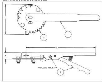
The lever-lock handle and throttling plate provide throttling notches every 10° for excellent manual control in balancing up to 90° or shut off service. The valve may be padlocked in any one of the positions including opened or closed by virtue of a locking hole located in the handle and lever.
