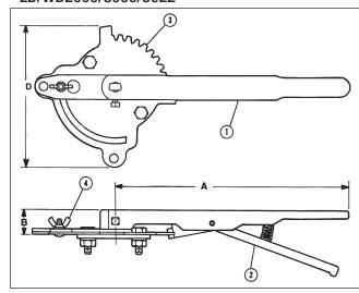
The position-lock can be used to set the valve in any position or as a memory stop so the valve may be reopened to the previous position. The valve may be padlocked in full open or full closed position.
