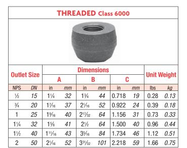
Each outlet size listed is available to fit any run curvature. Threaded ends are in accordance with ANSI/ASME B1.20.1. Design per MSS-SP-97.
