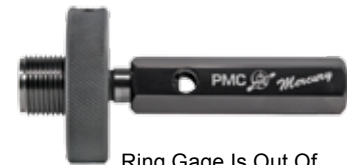
Ring Gage Is Out Of Tolerance If The HI Limit Portion Enters The Ring More Than 1 1/2 Turns
