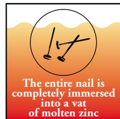
Maze **STORMGUARD**® NAILS have passed the ultimate test with flying colors – over 85 years of field service with a record unmatched by any other zinc-coated nail producer. No wonder builders and contractors say that **STORMGUARDS**® are the best steel-based nails on the market – economical, easy driving, and especially designed to properly apply all types of modern roofing, siding, trim and decking.
