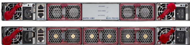
Arista 7280R3 1RU Rear View: Front to Rear airflow (red) AC Powered
