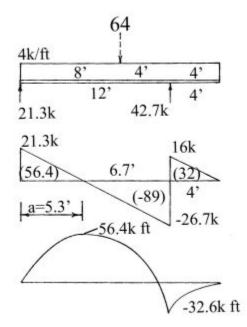
24. Using the simplified maximum horizontal shear stress formula for a steel I-beam, calculate the maximum horizontal shear stress in the steel I- beam. Determine the maximum vertical shear force from the beam diagrams. Use either the maximum positive value or the maximum negative value (whichever is larger) to calculate the maximum horizontal shear stress in the steel I-beam.
