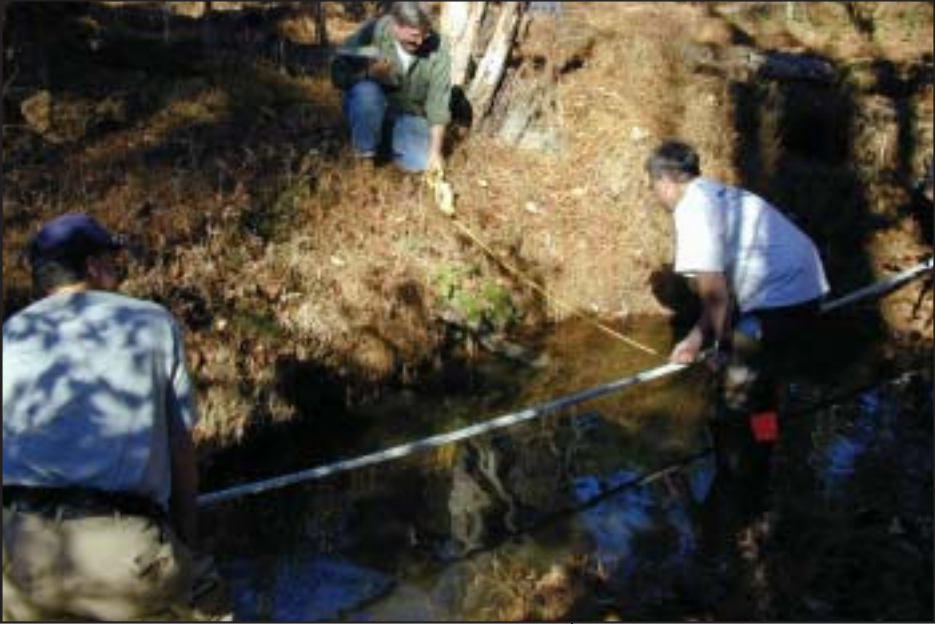
Figure 2.8 Field measurement of radius of curvature
