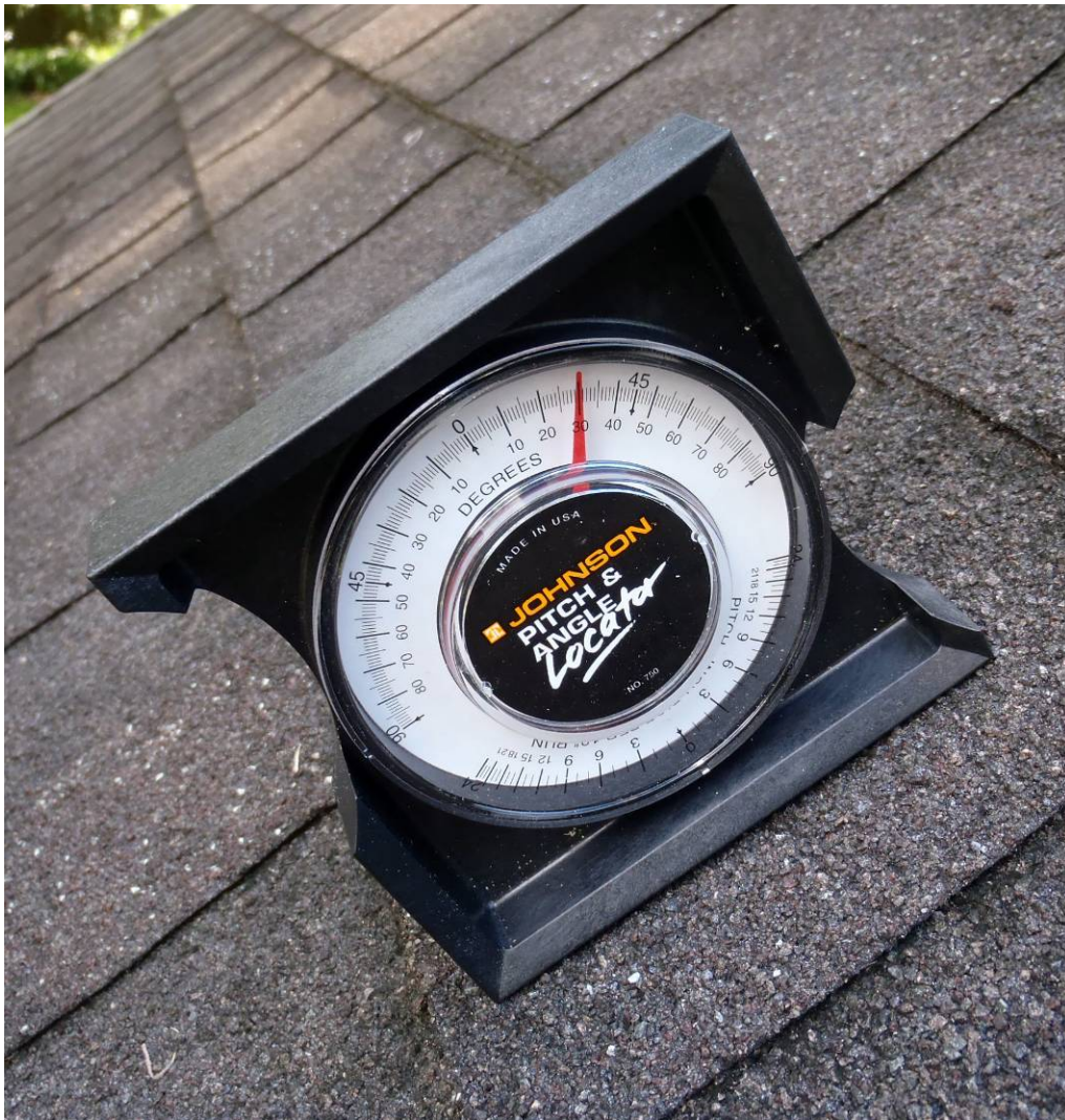
Inclinometer showing 30° roof angle
