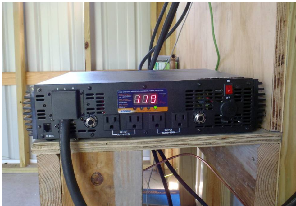
The front panel of the SunForce Inverter has four 120-volt AC outlets, one 12-volt DC outlet, and one wired 120-volt connection point (the large cable on the left side of the photo)
