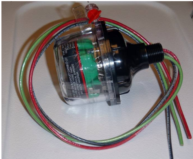
Surge protector and shown mounted
