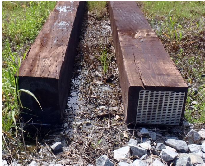
Figure 17 - A tie using a gang nail plate to control splitting during the curing process
