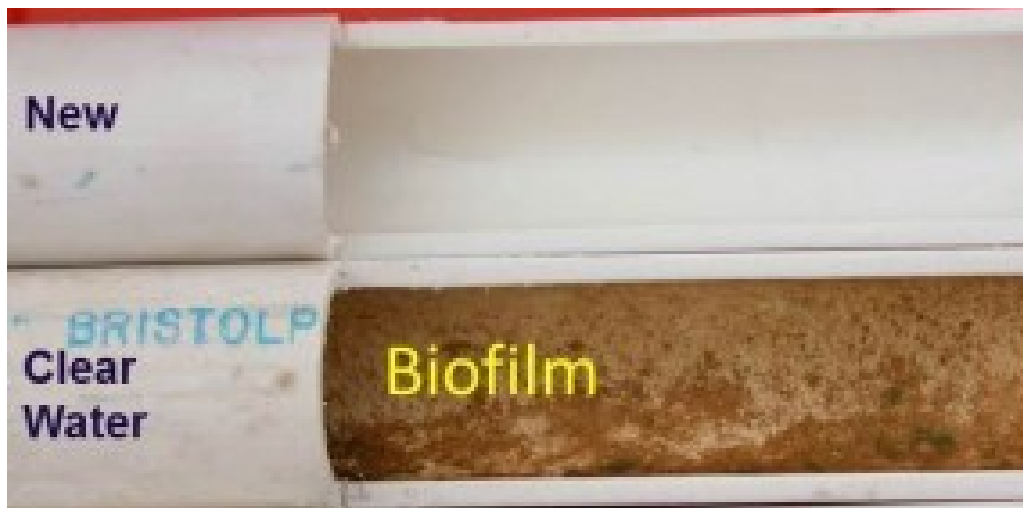
Figure 22: Brand new small PVC pipe (top) and pipe that was in service with brown biofilm growth (bottom).
