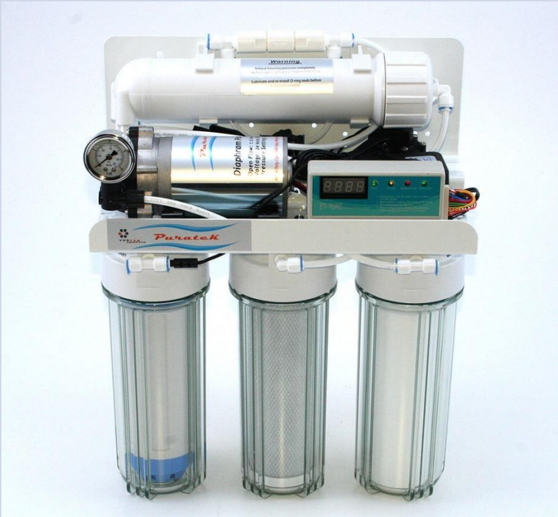
Figure 14: 4-Stage 100 gpd RO Water System with (3) prefilters (carbon and sand) at the bottom, a booster pump (silver) and a RO De-Ionizing Filter (white).
