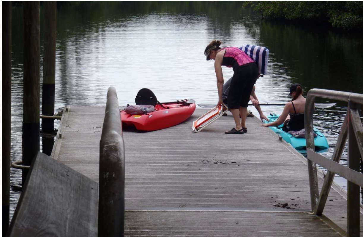
Figure 21 – A floating dock with a ramp from the pier to the dock makes for easy launching of kayaks and canoes
