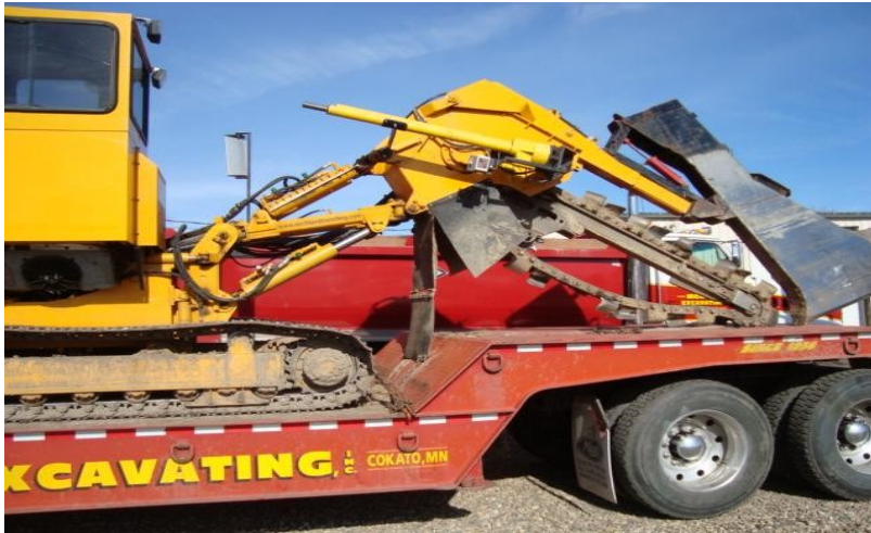
Figure 15 Heavy duty Minnesota agricultural chain trencher.
