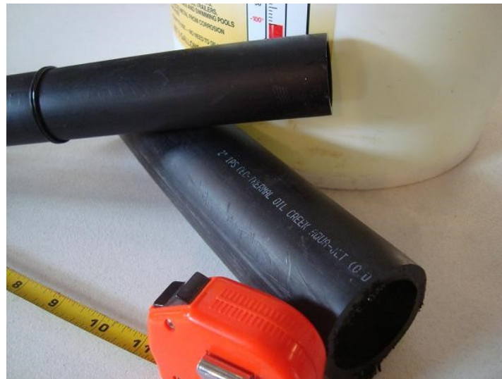
Figure 18 2in. HDPE loop material labeled 'Thermal' under a 1.25in. loop with a butt fused joint. Both rest against a 5-Gal. bottle of propylene glycol.
