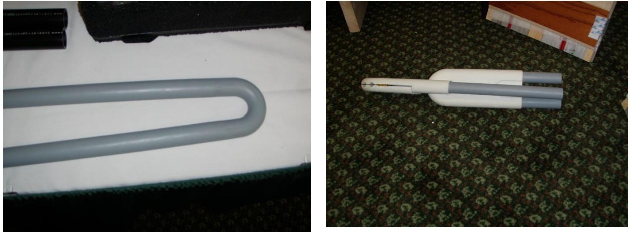
Figure 11 Left: PEX pipe molded U-bend. Right: 4 pipes in a hole, double PEXa U-bends.
