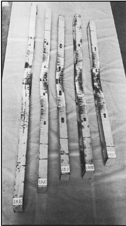
Photo No. 16 - Laterally buckled beams
