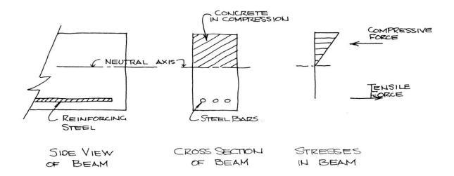
The compressive force is acting over the entire face of the concrete beam above the neutral axis. The maximum stress (in this design assumption) in the concrete occurs at the extreme fiber – the top of the beam and there is zero stress at the neutral axis. The tensile force is assumed to act only at the location of the reinforcing steel.
