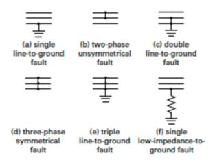
What fault is the most severe and determines the rating of the protecting circuit breaker?
