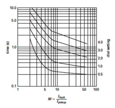
Analysis of a three-phase fault short circuit at the fault location on the 11 kV bus shown in the diagram results in a current on the 33 kV bus of 2300 A. The relay must operate at 2.0 s.
