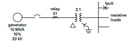
The relay has the characteristics shown on the graph with a minimum pickup current of 400 A.
