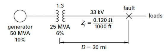
A fault occurs at the location indicated. What is most nearly the magnitude of the short-circuit current?
