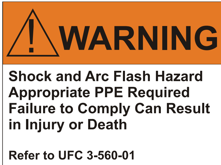
Figure 2-1 Typical Arc Flash Warning Label
