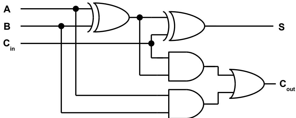
28. The logic diagram shown above is for a full adder. For an input of A = 1, B = 1, C<sub>in</sub> = 0, the output will be \_\_\_\_\_.
