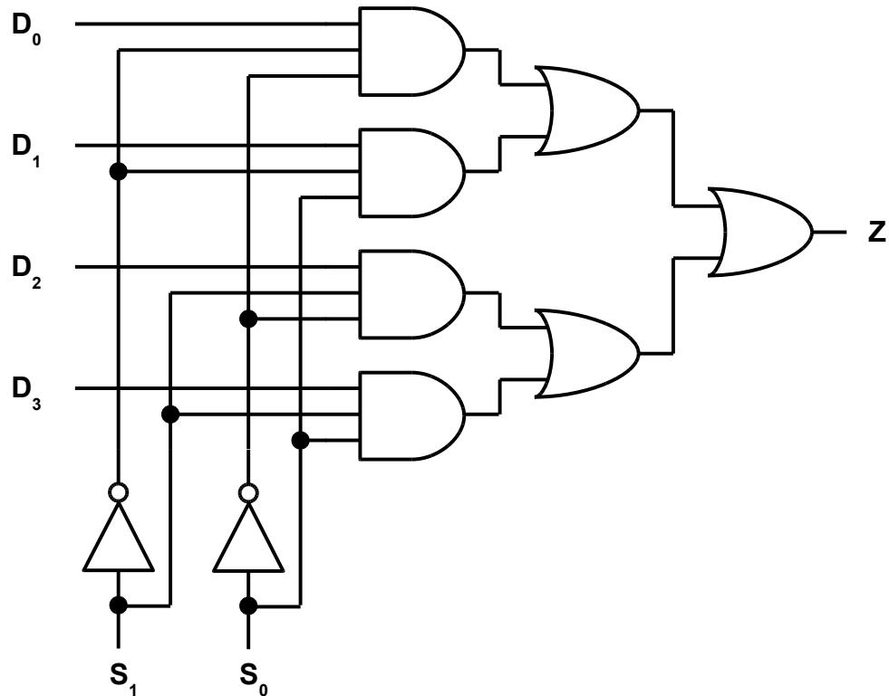
24. For the 4-to-1 multiplexer shown above, what input on the data select lines  $S_1S_0$  will route the input  $D_2$  to the output  $Z$ ?
