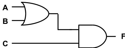
17. The combinational logic diagram shown above produces the expression \_\_\_\_\_.
