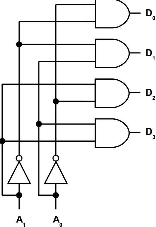
19. For a 2-to-4 decoder shown above, an output of  $D_3D_2D_1D_0$  of 0100 would result with an input of  $A_1A_0$  of \_\_\_\_\_.
