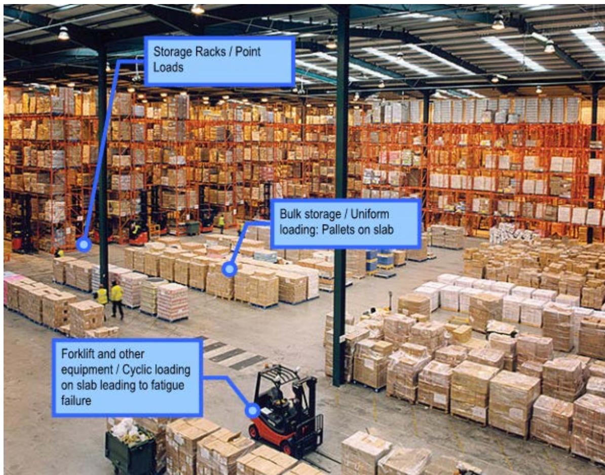
Fig. 24b - Typical loads on slabs
