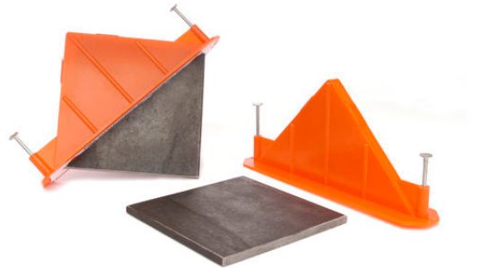
Fig. 37– Insert at edge of construction joint set into first concrete pour, with second concrete pour to follow. Square dowels shown to be placed at a construction joint placed in insert that was set into first concrete pour, with second concrete pour to follow ( https://www.pna-inc.com/products-designs/diamond-dowel-system )
