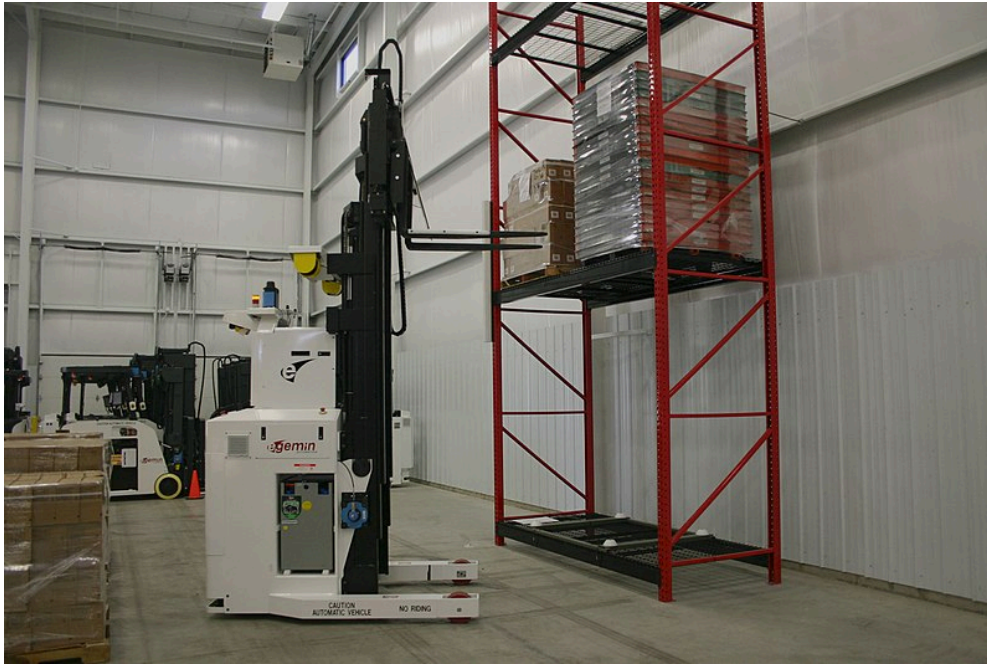
Fig. 13- Stacker with outrigger feet
