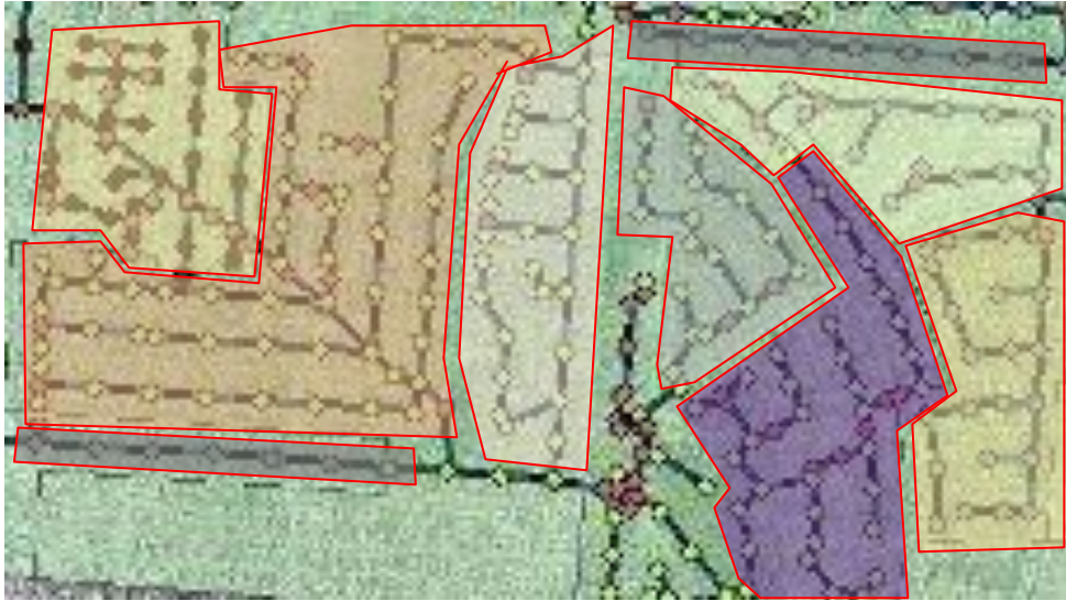
Figure 22: GIS map with sewersheds highlighted in red. When defining a sewershed, it is helpful to make the area as large as possible with the flow still going through a single path such as a manhole or lift station.
