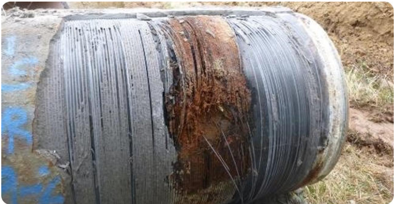
Figure 19: A section of prestressed concrete cylinder pipe (PCCP) with wire damage discovered by internal electromagnetic scanning.
