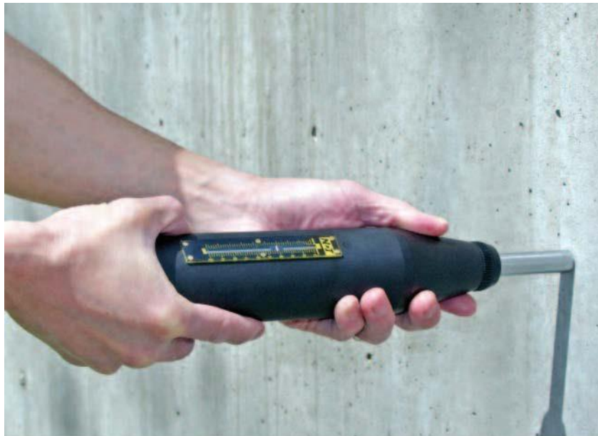
Figure 22: An example of a test hammer instrument that gives an estimated strength reading in psi (MPa).
