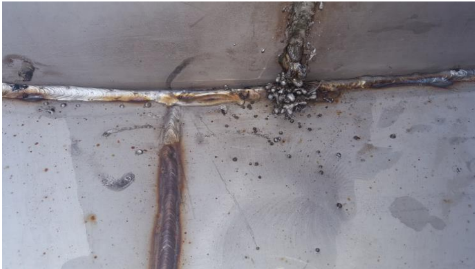
Figure 44: Stainless steel welds with excessive slag and discoloration. Also, note the orange specks of carbon steel contamination.
