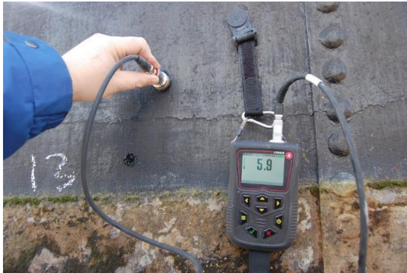
Figure 16: Steel thickness measurement with an ultrasonic thickness gauge. In this example, the design thickness was 1/4" with a 1/16" corrosion allowance, so the minimum thickness is 3/16", or 0.19". This gauge is reading 5.9 mm, or 0.23", which is above the minimum and therefore acceptable. Note the conversion: 1 inch = 25.4 mm.
