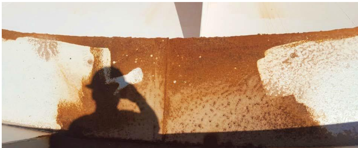
Figure 40: A blasted surface after 5 days, with an area in orange that was not prime coated and has started to corrode.
