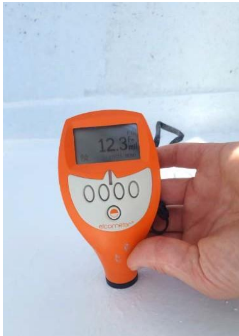
Figure 17: Coating thickness measurements with a coating thickness gauge that reads in mils dry film thickness (DFT). One mil is one-thousandth of an inch thick. Submerged carbon steel is often coated a minimum of 12 mils DFT.
