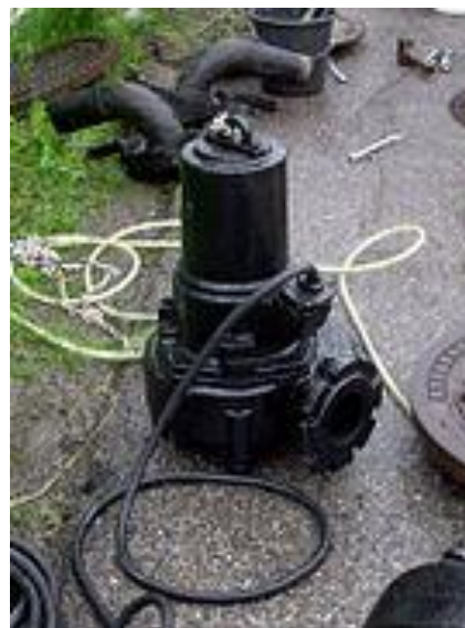
Figure 8: Examples of submersible centrifugal pumps. These types of pumps are common for wastewater wet wells and sumps. https://commons.wikimedia.org/wiki/File:NS_non_clog_submersible_pumps.jpg by Mukund275, CC BY-SA 3.0 https://commons.wikimedia.org/wiki/File:Tauchpumpe_Abwasser.jpg by Dergreg, CC 1.0
