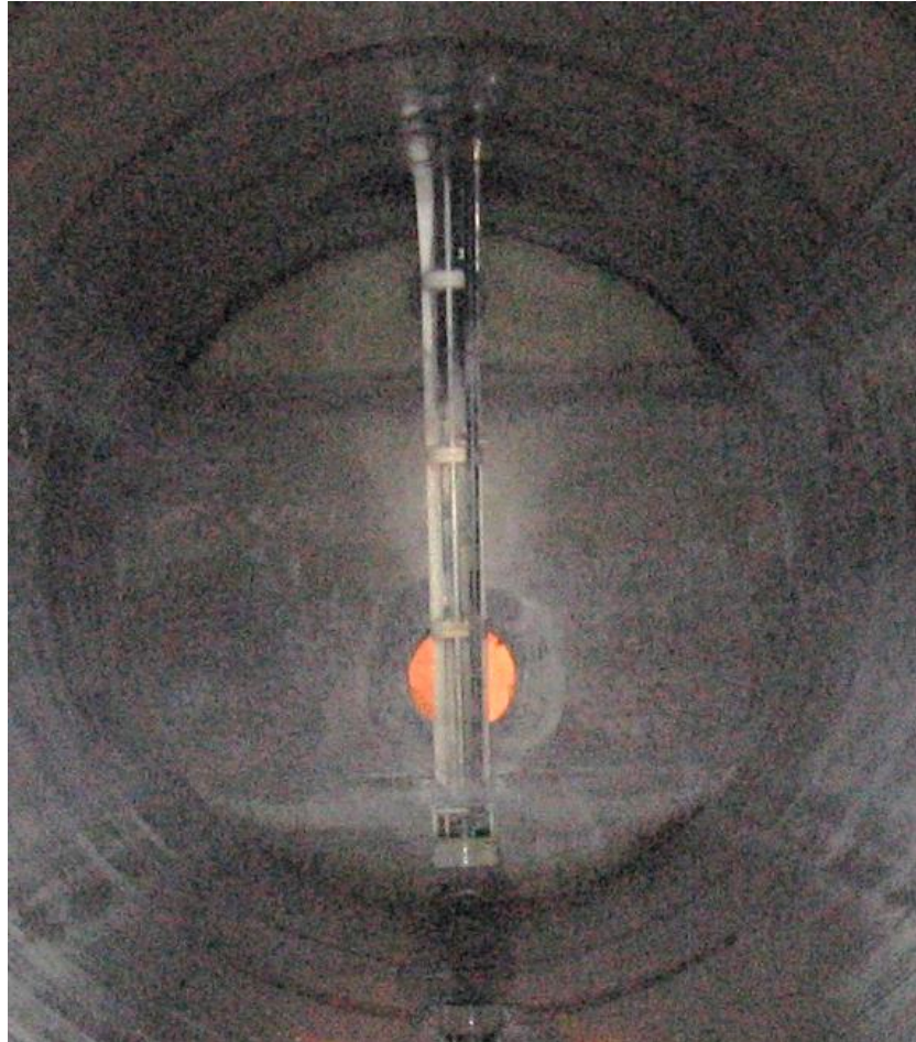
Figure 6: A vertical suspended column centrifugal pump for chemical pumping. The motor is mounted safely above the tank. The impeller is submerged near the bottom of the tank. A small discharge pipe rises to the left of the enclosed vertical shaft.
