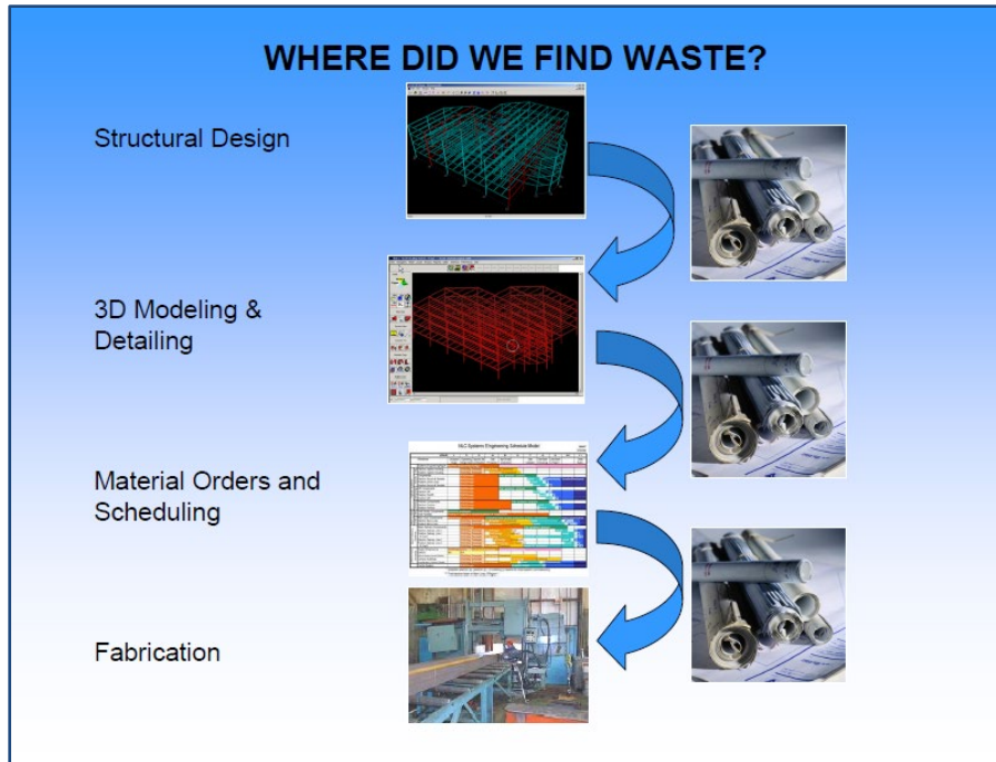
Figure 8 Illustration of analog process in steel fabrication and depiction of waste (AISC)
