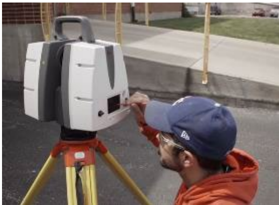
Generating Cloud Points for a 3D Model Picture provided courtesy of Livers Bronze
